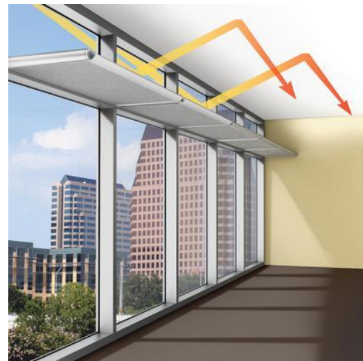
fig 8: design of overhangs scatters the light entering the space in a better way and provides glare free space
